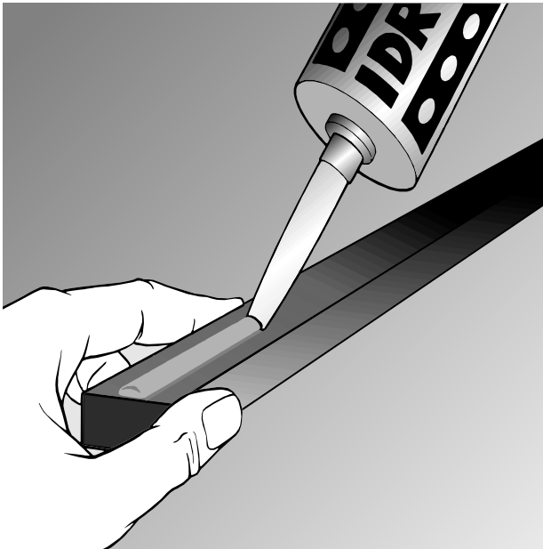
Apply the MS-polymer-based adhesive evenly on the Idrostop or directly to the substrate.
